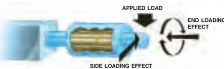
The Weigh Bar is a fully electronic method of weighing loads. A steel bar, fixed at one end, bends while electrical current is run through strain gauges fixed on the top and bottom of the bar. The change in current is translated by the indicator into a weight reading.
